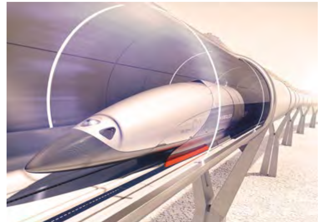
ABOVE Render of the Hyperloop's Maglev capsule in its low-pressure tube
